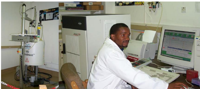
300 MHz NMR facility and technician in the University of Botswana (Photo courtesy of Berhanu Abegaz, former Director of NABSA and IOCD Senior Advisor)
